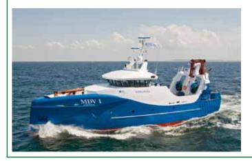
Hoekman Shipbuilding and Padmos have designed and build a revolutionary, innovative and sustainable trawler. The special hull design is like the shape of a whale: a sharp bow in the front, a big belly for the fish hold in the middle and a strong tail/propellor at the stern. These lines gives her less resistance, more propulsion power to tow the nets and good stability and sailing speed.
